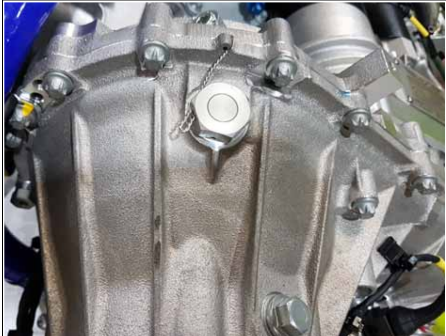
Fig. 6.48 Lock wiring the oil filler screw
