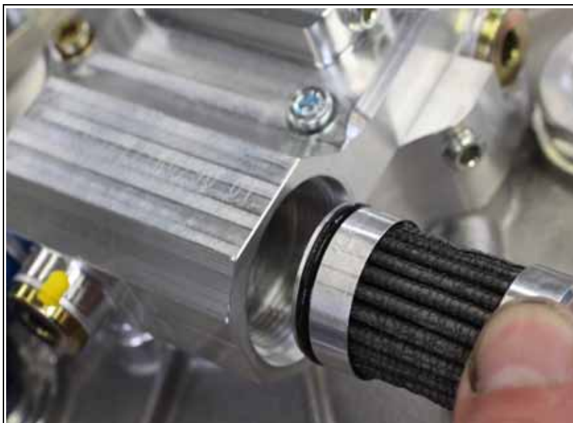
Fig. 6.45 Mounting direction of the oil filter
