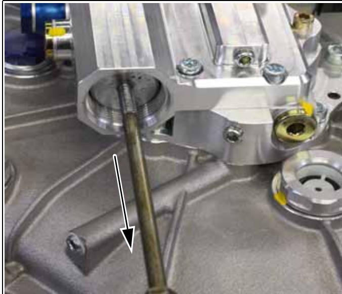
Fig. 6.44 Removal of gearbox oil filter
