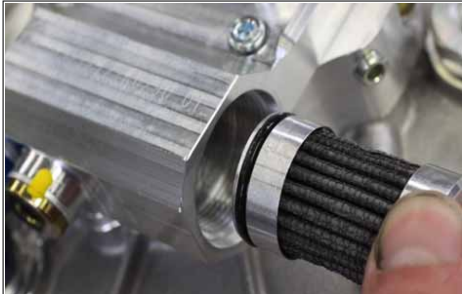
Fig. 6.19 Mounting direction of the oil filter
