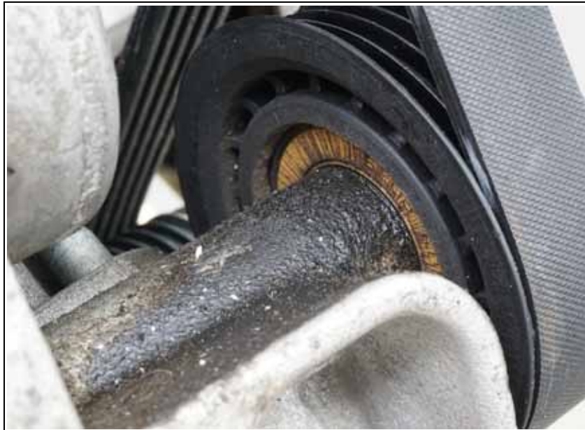
Fig. 6.61 Inspecting the V-Ribbed Belt Pulleys NOT OK - needs to be replaced
