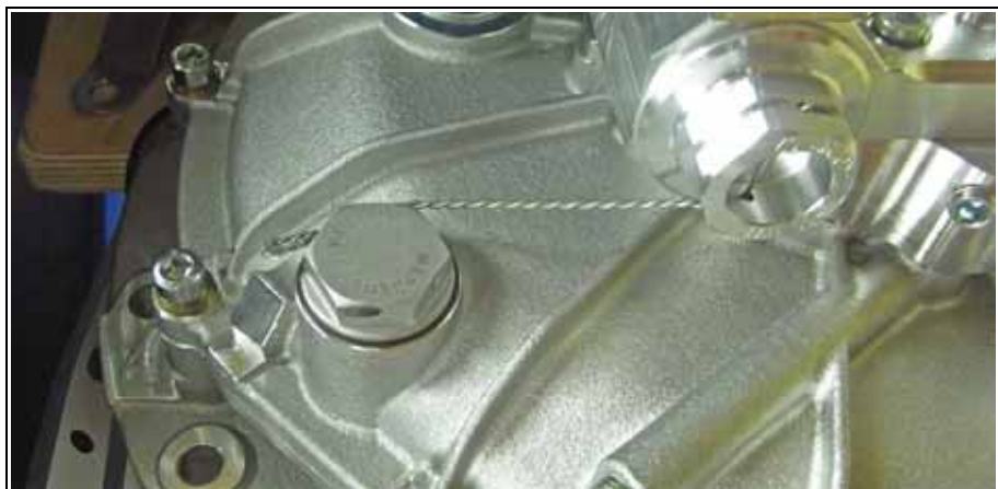
Fig. 6.21 Lock wiring between oil drain plug and oil filter cap
