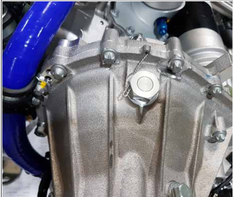
Fig. 6.24 Lock wiring the oil filler screw
