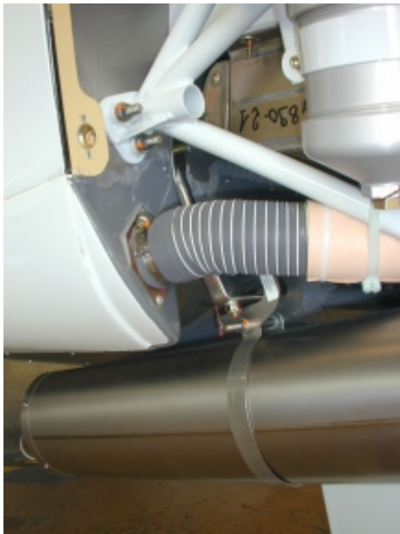
Fig. 78.2d Fixing point of exhaust system on firewall
